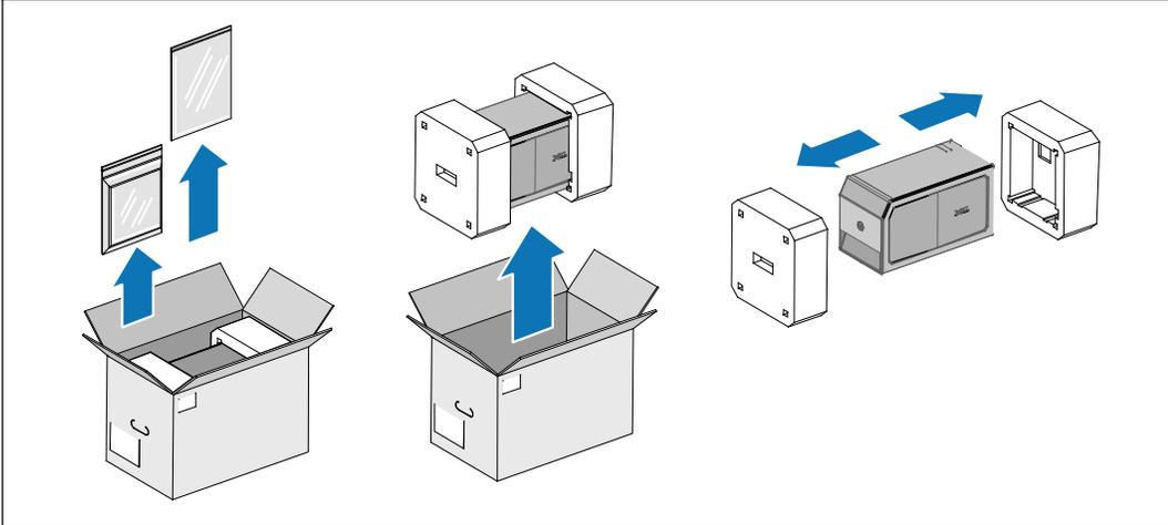
**1** Unpack the External Battery Module (EBM).
